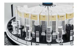
the respons<sup>®</sup>910 is also a good example for efficient, highly developed design. The respons<sup>®</sup>910 is the only analyzer in its class with a multifunctional arm that integrates clot detection and crash sensor, liquid-level detection and pipetting of sample and reagent. The instrument is user-friendly as well since all components are almost maintenance-free.
